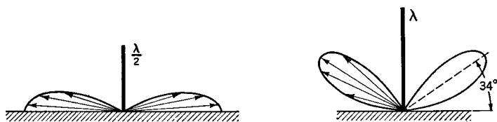
FIG. 8 E. Radiation patterns from vertical Marconi antennas
